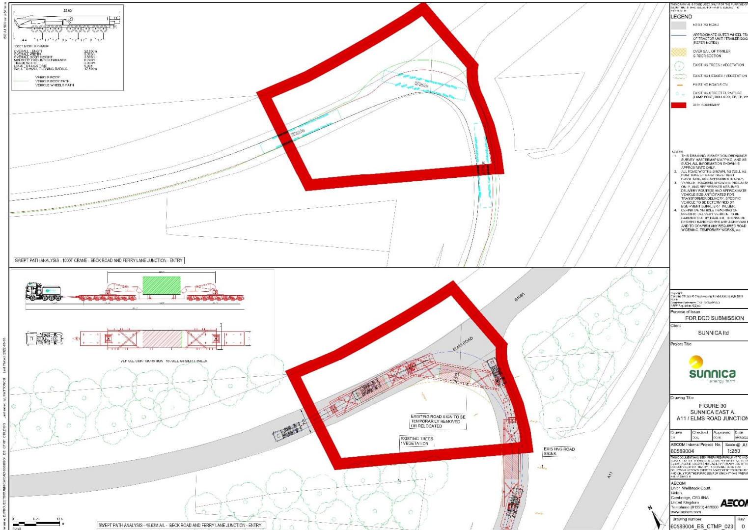
Figure 30: Swept Path Analysis – 1000T Crane and 46.63m AIL – A11 Northbound Off-Slip/Elms Road Junction
